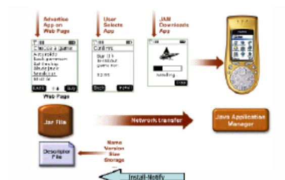
Figure 12 Over the air (OTA) provisioning (source: Nokia [6])
